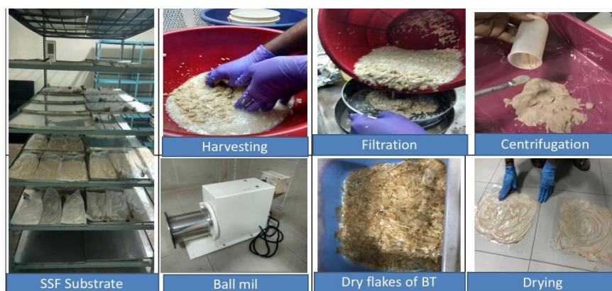
Fig. 22: Steps involved in production process of Bt through SSF method fermentation
